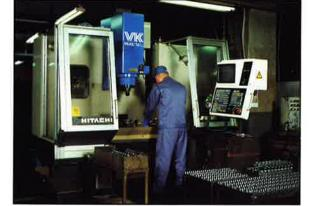
The SKB receivers are milled from a solid block of steel by a multi-head Hitachi robotic machine tool. This state-of-the-art equipment insures precise tolerance in critical components.
