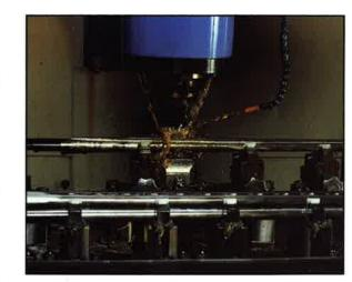
Ventilated ribs are attached and aligned with precision computer controlled equipment for correct point of impact.
