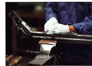
Once the initial phase is completed by the computer operated milling machines, the master gunsmiths begin their work of fitting, assembling and polishing the critical components of the receiver, barrel group and forend iron. The engraving is then rolled onto the polished metal prior to hardening and final finish.
